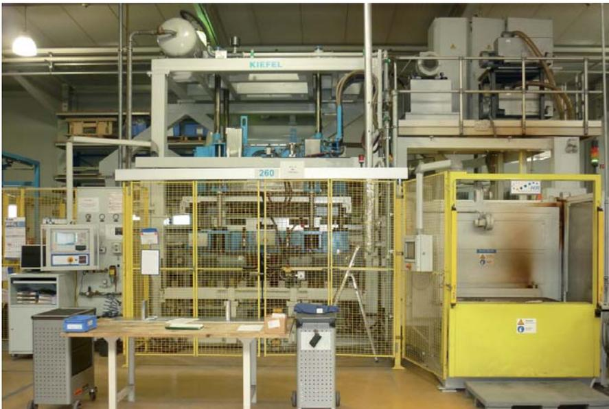
Picture 2 : A deep-drawing machine of Kiefel is used at Jacob Composite for the production of the trimparts
